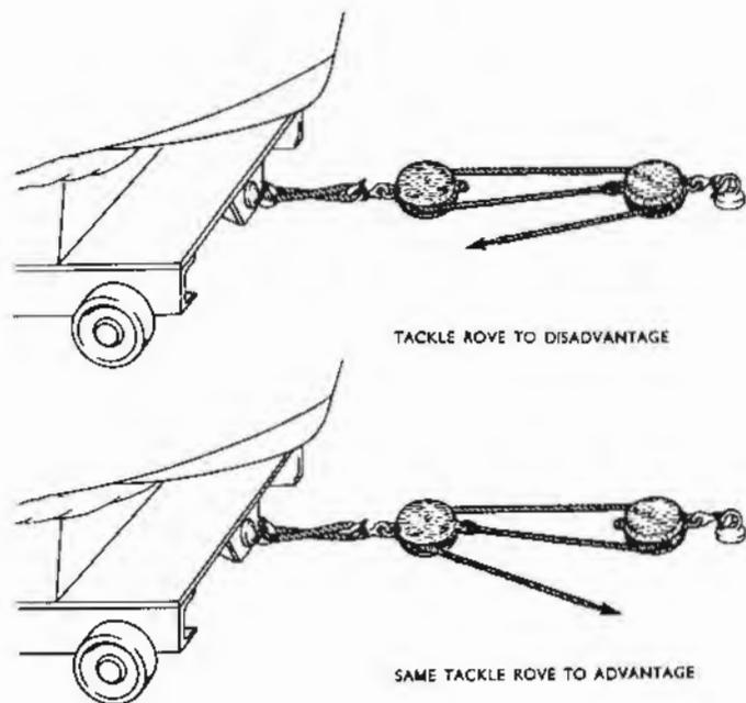
FIG. 8-8. Reeving a tackle to advantage and to disadvantage
