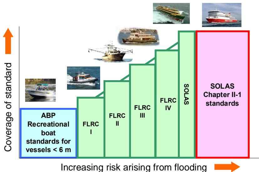
**Figure 2—Illustration of how the Flooding Risk Categories provide a graded approach to the requirements for buoyancy and stability after flooding**
