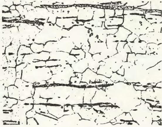
FIG. 1—21. Photomicrograph at 100X showing typical structure of wrought iron parallel to the direction of rolling. White areas are the highly refined iron matrix. Dark gray elongated lines are iron-silicate slag filaments. (Courtesy, A. M. Byers Company.)
