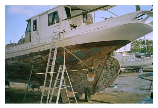
A similar process of measuring off a triangular frame of known dimensions and referenced to known locations on the hull is also used to establish the profile shape of the bow and stern. The pictures below show this being done for the bow of TRIBAL WARRIOR (originally MINA, an 1899 Thursday Island lugger) and the stern of VIKING.
