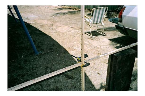
If the boat is lying on its side I set up the stations at right angles to the side face of the keel. This introduces an unwanted source of error and is far from ideal, but sometimes you don't have any choice. The pictures below illustrate what I mean; they show the abandoned hulk of VIKING, looking very forlorn.
