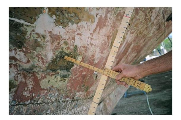
The offset in this picture would be recorded as 10-0 (ten inches exactly) at datum D2-0-0 (the two foot mark on the diagonal batten). Note that it's *very* important to be consistent about which edge of the batten you measure to! To avoid mistakes I always measure to the edge that's marked with the graduations.
